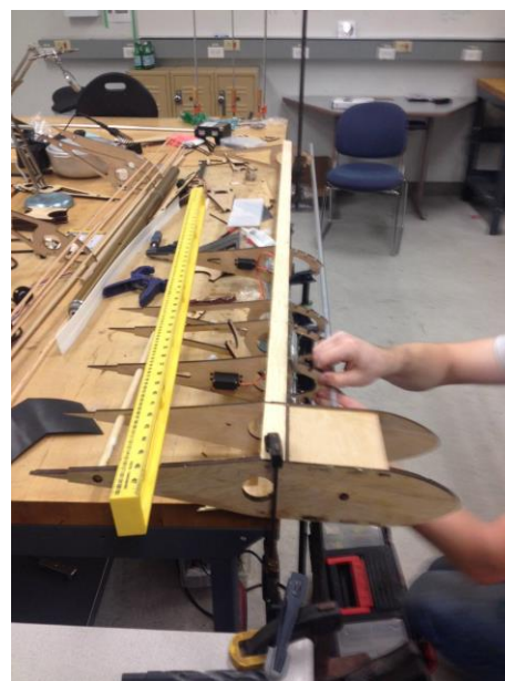
Figure 24: Bonding the ribs to the spar caps
