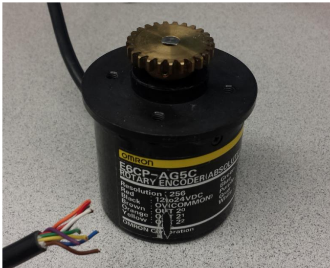
Figure 16: Absolute encoder with grey code output wires
