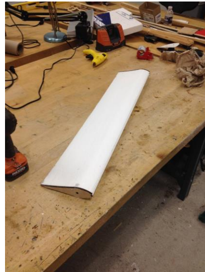
Figure 27: Styrofoam tail-wing core
