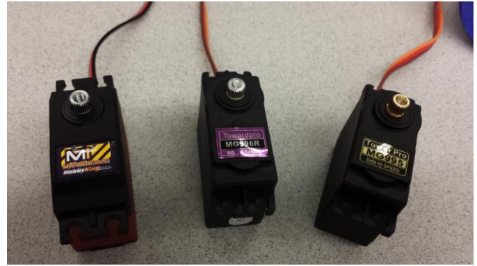
Figure 30: The 3 servos tested (From Left: HobbyKing MI, MG996, MG995)
