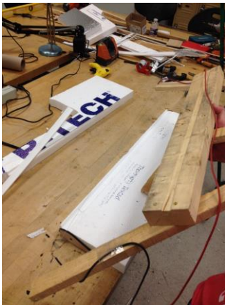
Figure 26: Hotwiring the Styrofoam-core tail-wing
