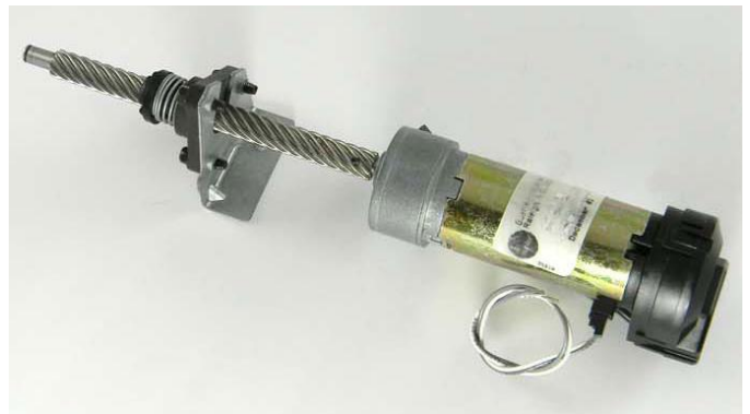
Figure 14: A DC motor with a lead screw
