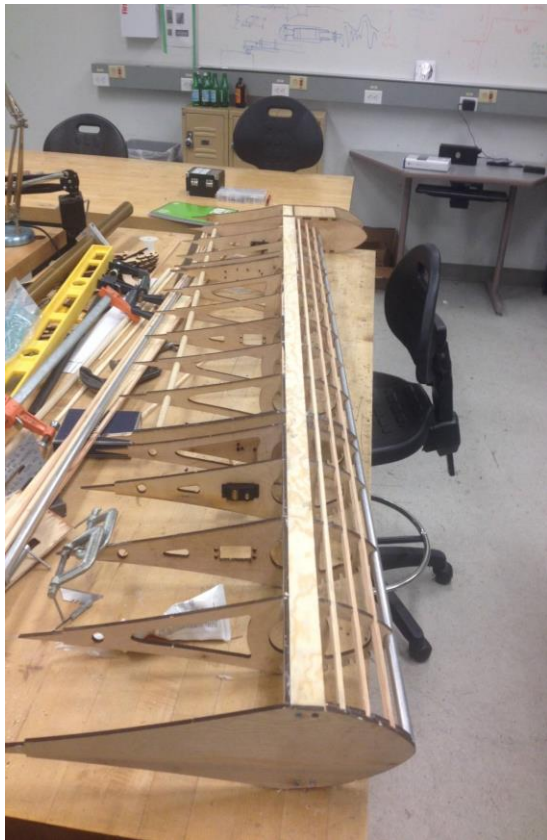
Figure 25: The main-wing skeleton
