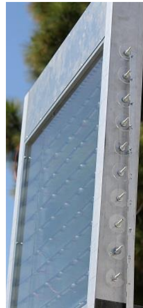
Figure 8: Side view of rotating rods used to control each row in the solar array.
