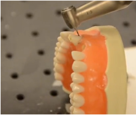
Fig. 9: The robot executing the trajectory on the incisor model
