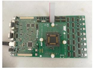
Figure 3: Atmel STK600 development board with mounted Atmel AT32UC3A0512 microcontroller.
